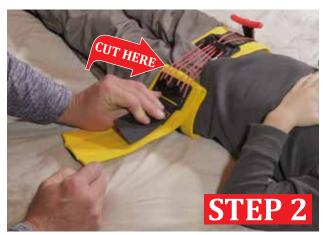
Fold Back the excess material and extend the loose end of the plate to the other side of the belt. Use this gap width between the two ends of the plates as a cutting guide.
